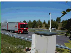
SASV provides high speed 140 weigh-in-motion (30 to Km/h) of vehicles with the purpose of detecting overloaded trucks. SASV uses 2 piezoelectric sensors and electromagnetic loop per lane. A video camera records the overloaded vehicle captures its registration plate.
