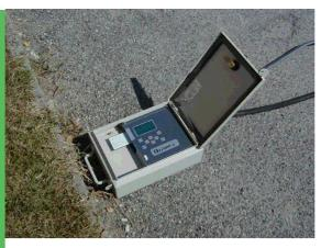
TENOR is a traffic classifier with 2 pneumatic inputs.
