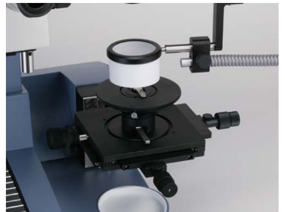
diffuser for shadow-free illumination
