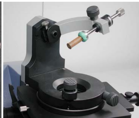
holder with plasticine for Ø 5, 10, 15 and 20 mm
