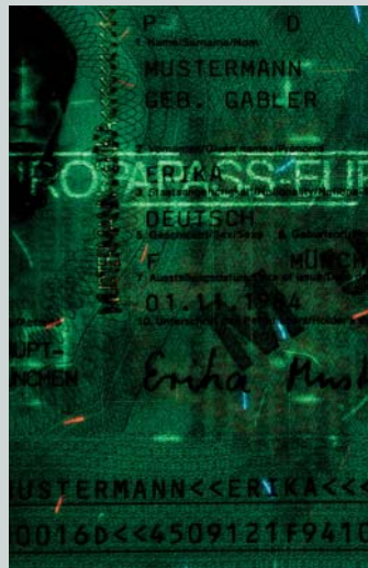
■ Hidden information in transmitted UV light in German travel documents.
