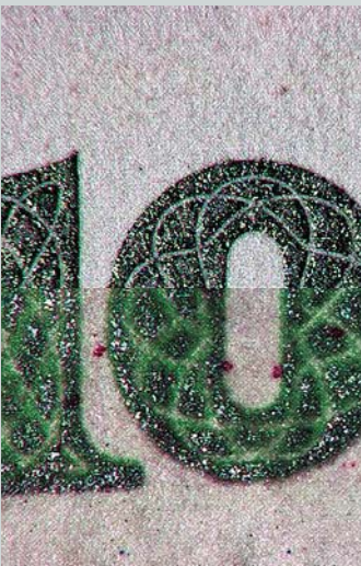
■ Horizontal split image of OVI. Above: Original, below: Forgery.
